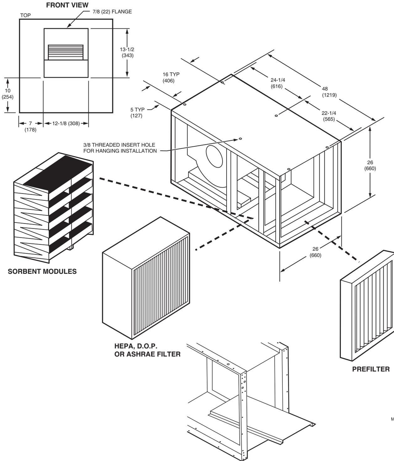
ALL MODELS, EXCEPT F116A1021 AND F116A2021, ARE EQUIPPED WITH A DISPOSABLE ALUMINUM SPACER. THE SPACER IS SUPPLIED TO ACCOMMODATE THE CPZ MODULES. IF YOU DO NOT USE THE CPZ MODULES, REMOVE THE SPACER. IF YOU USE TWO SETS OF CPZ MODULES (4 MODULES) IN A THREE STAGE CABINET, YOU WILL REQUIRE AN ADDITIONAL SPACER. SAVE A FEW SPACERS THAT ARE NOT NEEDED TO ACCOMMODATE FUTURE NEEDS.
